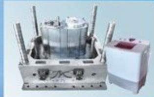
WASHING MACHINE MOULD
